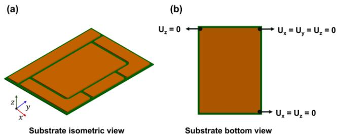
Figure 3. (a) Substrate 3-D and (b) mechanical boundary conditions for warpage simulation.
