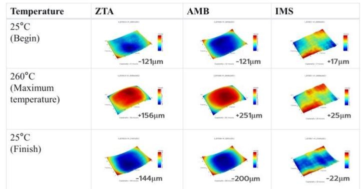
Figure 7. Evolution of warpage maps for representative ZTA, AMB, and IMS substrates at key temperatures (initial 25 °C, peak 260 °C, and final 25 °C) during a simulated reflow cycle
