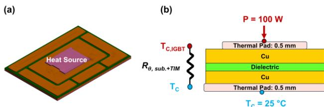
Figure 2. (a) 3-D finite element model and corresponding mesh structure used in the analysis. (b) Boundary conditions for thermal resistance estimation and the equivalent thermal resistance circuit.
