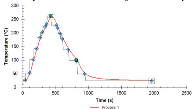
Figure 4. Temperature profile used for warpage measurement
