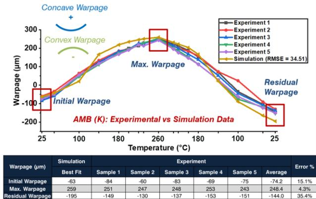
Figure 8. Comparison of warpage simulation versus five experimental measurements for the AMB-K substrate.
