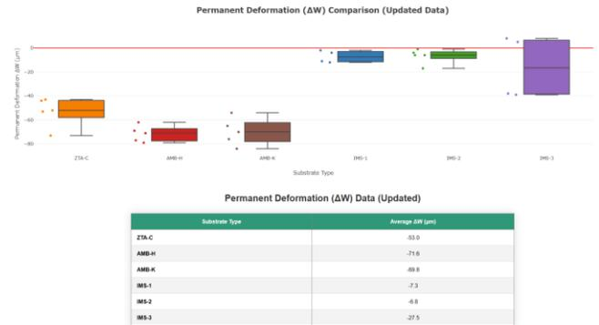
Figure 6. Box plot of permanent deformation ( $\Delta W$ ) for all substrate types following a simulated reflow cycle.
