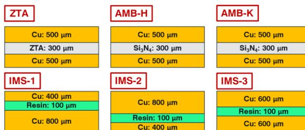
Figure 1. Schematic cross-sections of the substrate stack-up designs: ZTA, AMB, and the three IMS configurations.
