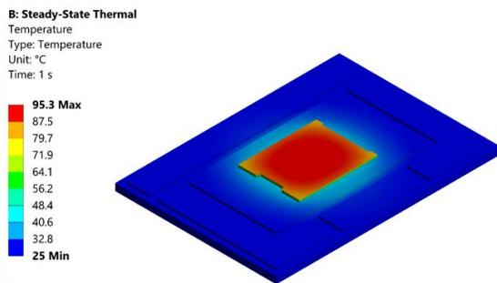
Figure 5. Simulated temperature distribution of the IMS-1 substrate from the steady-state thermal analysis.
