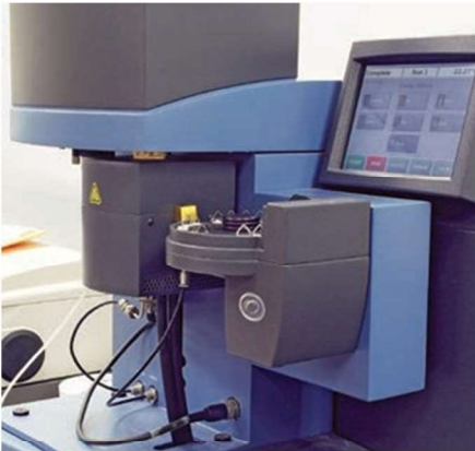
Thermogravimetric Analyzer (TGA) – Measures the stability of our dielectrics at high temperatures, baking the materials at prescribed temperatures and measuring weight loss.
