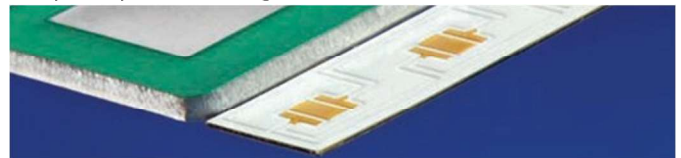
Photographic example of UTC versus a standard 0.062" (1.57mm) aluminum substrate.
